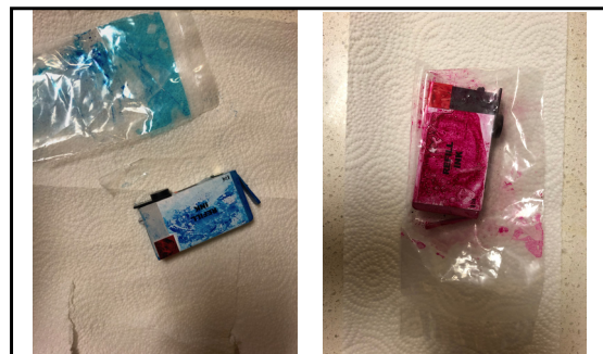
NON-HP CARTRIDGE INK LEAKAGE
