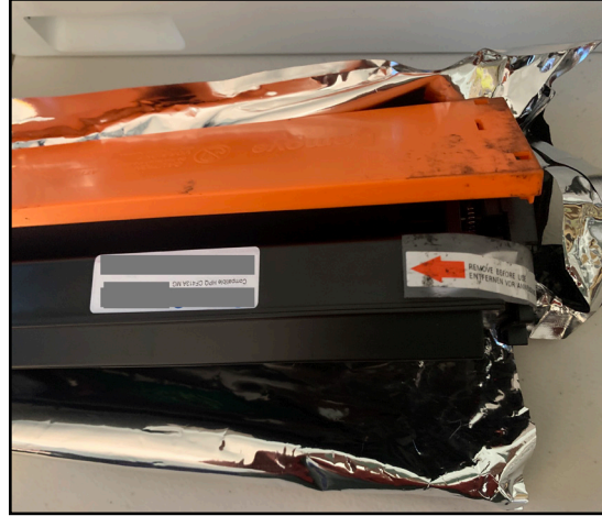
CARTRIDGE LEAKING AT UNPACKING
