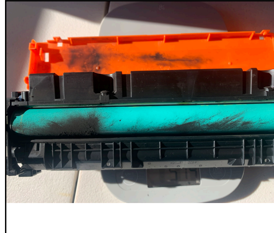
CARTRIDGE LEAKING AT UNPACKING
