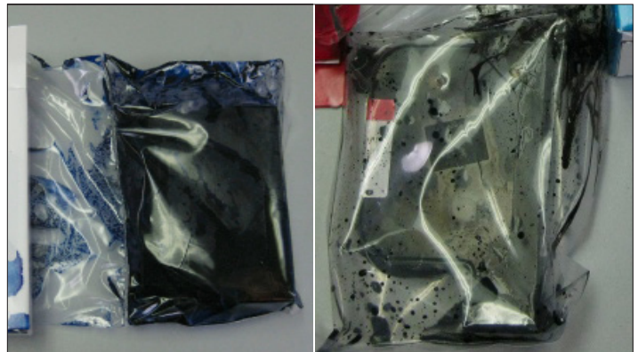
Figure 2: Refill Supplier cartridges Dead on Arrival (DOA) due to significant leakage
