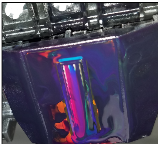
PRINthead DAMAGE CAUSED BY NON-HP INK
