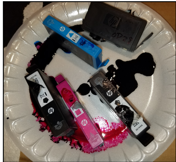
NON-HP REFILL CARTRIDGE: SEVERE INK LEAKAGE DURING REFILLING PROCESS
