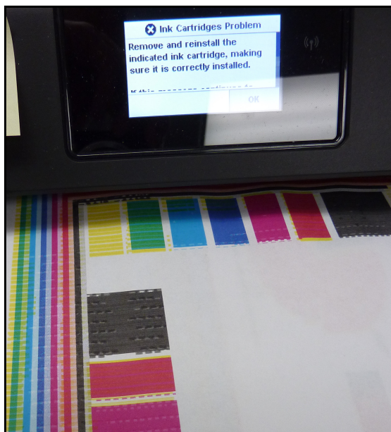
NON-HP: UNUSABLE PRINT QUALITY DUE TO PRINthead DAMAGE
