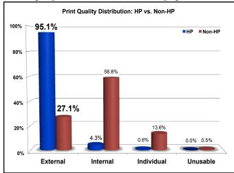
HP cartridges produced only 4.9% Limited Use pages (with PQ categorized as either Internal Use, Individual Use, or Unusable); whereas, Limited Use pages accounted for 72.9% of non-HP brand output. Of the non-HP brand Limited Use pages, 56% exhibited print quality defects such as vertical and horizontal Streaks and Ghosting.
