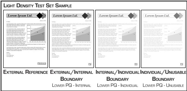
Examples above are the boundary samples from two of the fifteen test sets.
