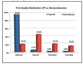
produced a total of 95.9% of print samples categorized as good for External Use. Comparatively, the remanufactured cartridges produced only 19.7% of pages that were good for External Use.
