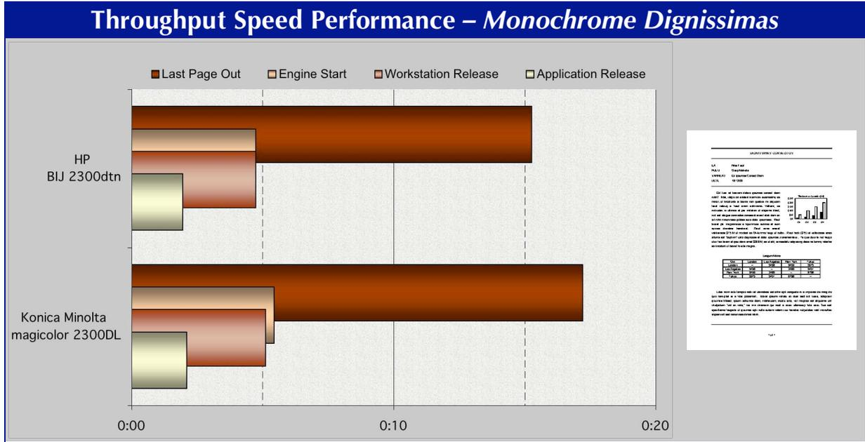
APPLICATION RELEASE for the printers was within 0.2 seconds, with the BIJ 2300 at 1.9 seconds and the magicolor 2300 at 2.1 seconds. WORKSTATION RELEASE on the BIJ 2300 occurred simultaneously with its ENGINE START at 4.7 seconds, faster than both the WORKSTATION RELEASE and ENGINE START of the magicolor 2300 at 5.1 seconds and 5.4 seconds, respectively.
