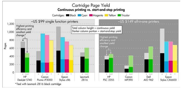
Page yields derived from typical start-and-stop printing are different from those measured when printing continuously. As shown in the charts above, the relative yield rankings of the printers tested change between start-and-stop printing and continuous printing. In both test groups, the HP printers tested demonstrated the smallest percentage change between continuous printing and start-and-stop printing.<sup>1</sup>
