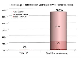
and Premature Failure cartridges (those with page counts of less than 80% of the average page count for all HP toner cartridges of that model, but not DOA) accounted for 11.7% of the remanufactured cartridges. For the average user, problem cartridges are disruptive, causing inconvenience due to a lack of reliability, which impacts and increases the overall cost of printing.
